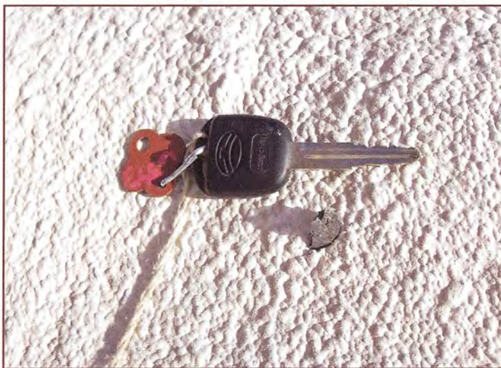
Figure 19 – Shell fragments still capable of severely wounding personnel were embedded in the foam of the structures, 80 to 100 yards away from impact.
